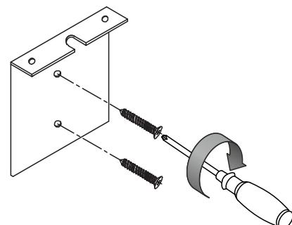
**GB** The wall plugs included are only to be used in brick- or concrete walls. If you have another type of wall you should buy the wall plugs required for that type of walls in your local DIY-store. All screw holes you drill in the wall in a bathroom should be sealed with silicone. We recommend that you put silicone into the screw hole before you insert the wall plug. Then you put silicone into the wall plug before you fix the screw into the wall plug.
